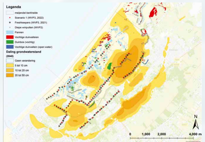
Drawdown of the shallow groundwater level due to the abstraction of brackish groundwater in the year 2040 (after ten years of operation), relative to the reference situation. Sensitive nature areas are shown in red (moist dune valleys) and green (moist dune forest).
