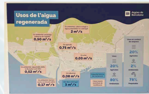
Flows of reclaimed water in Barcelona. The reclaimed water is amongst others used to supply the Llobregat hydraulic barrier and to provide irrigation water to farmers via a managed aquifer recharge system (pilot in Horizon Europe project MARCLAIMED).
